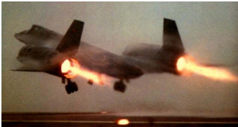
Figure 2. Shock diamonds shown expelled from the SR-71's J58-1 twin-engine in airborne position when afterburner is used ( http://www.wvi.com ).
