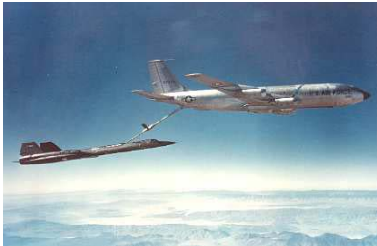
Figure 5. The special tanker KC-135Q was delivering special JP-7 fuel streams to the SR-71C no. 61-17981 via its receptacle during a flight training ( http://www.wvi.com ).
